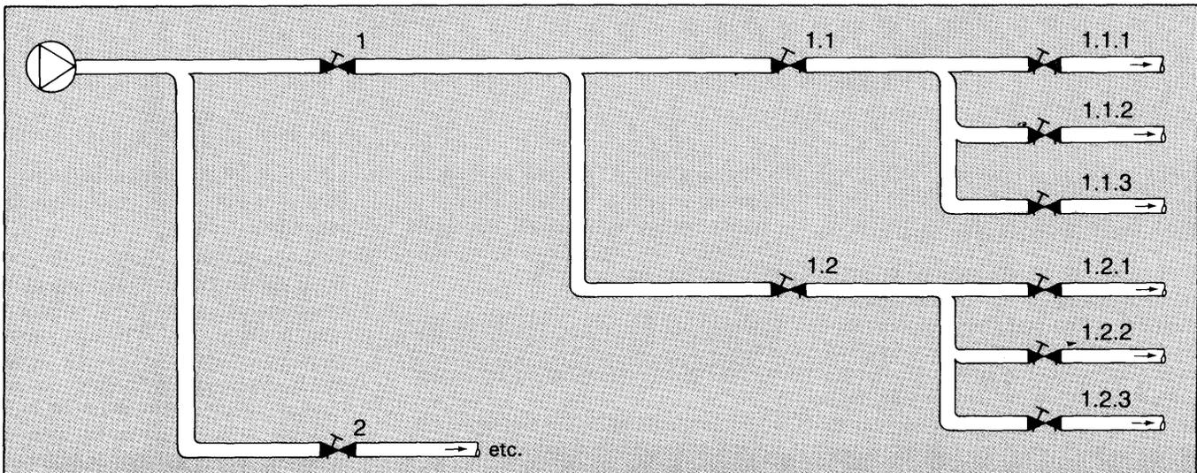
There, all the valves are measured after, for example: valve 1.1. The flow quota for each valve is noted.
